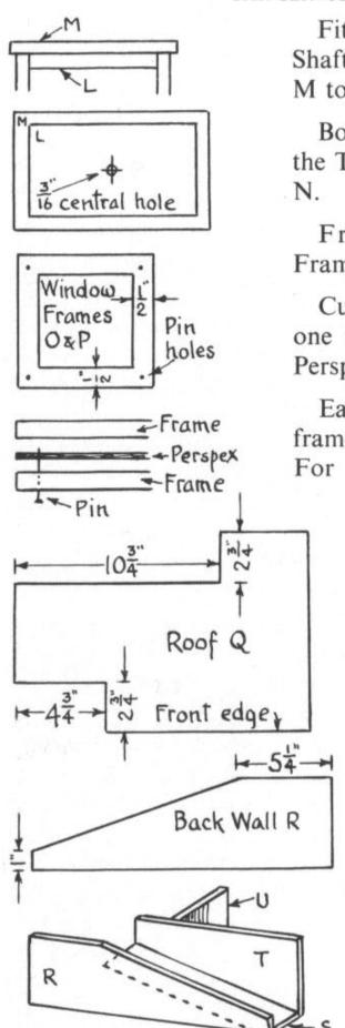
Fit the Inside Top L inside the Shaft top. Pin the two Tops L and M together.
