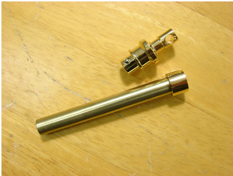
Holder Cup Pressed Into Tube Insert
