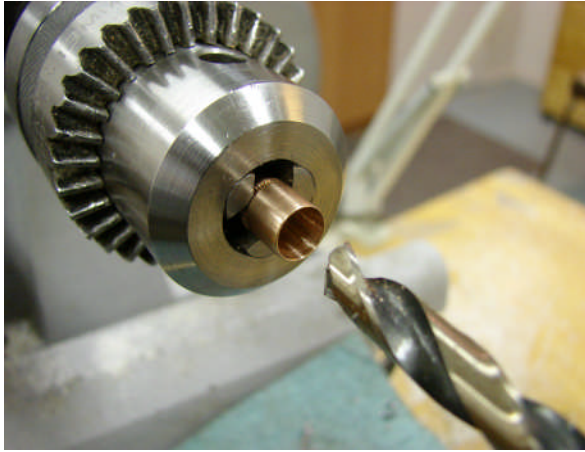
Drilling 7mm Hole
