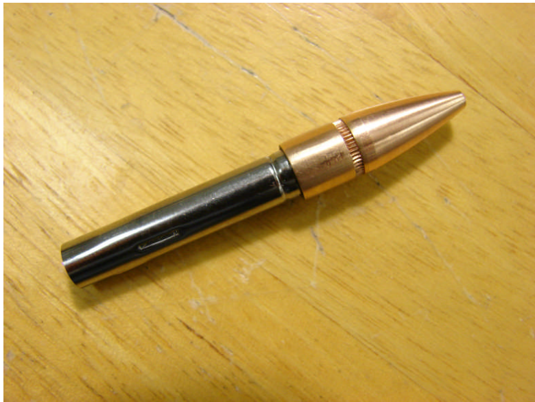
Transmission Pressed Into Bullet Tail
