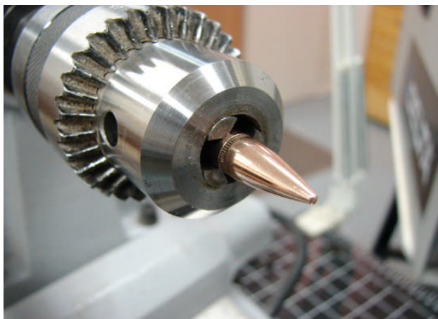
Bullet Installed In Drill Chuck
