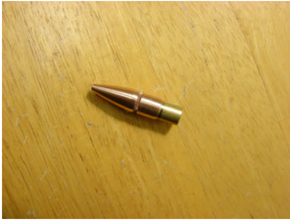
Cut Tube Flush with Bullet Tail
