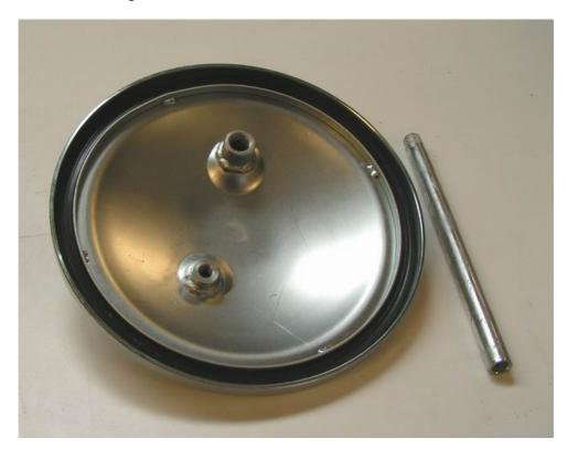
When you look on top of the lid there are 2 threaded entrance holes, one is 3/8" BSP (the bigger of the two) and the other apparently 1/4" BSP (more on this later). I wanted to use the bigger (3/8" BSP) for the air inlet.
