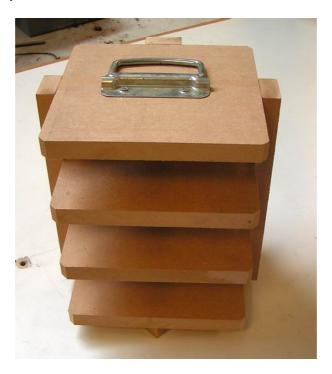
I have fitted a diagonal piece to the bottom which locates it in the dished bottom and a handles for ease of handling.
