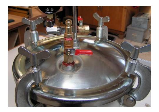
The cut off valve fitted can also be used to lower the pressure in the pot if you go a bit higher than you wanted to, whilst the inlet hose is still connected.
