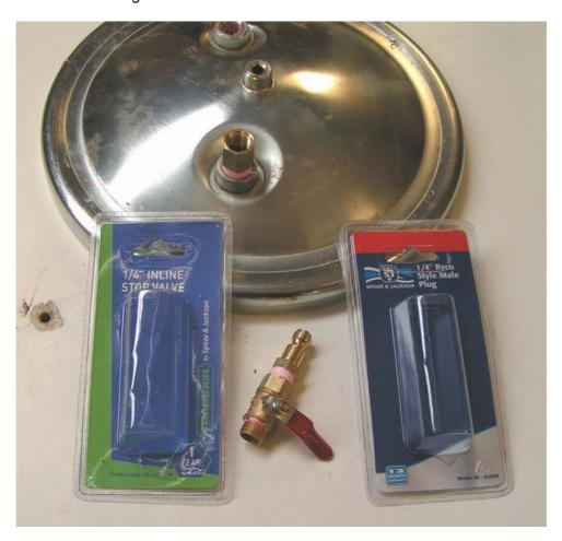
I then fitted a 1/4" BSP cut off valve and as my air system in the shed uses Ryco fittings, a Ryco male plug.
