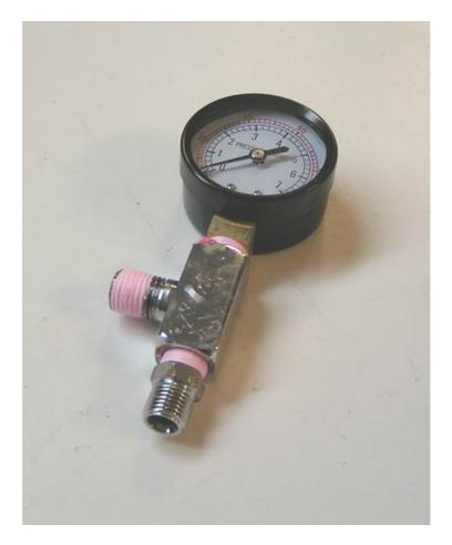
Here we have the original right angle fitting that held the regulator fitted back to the T piece with the pressure gauge mounted directly to it. Also we have a 1/4" BSP cut off valve fitted to the other side of the T piece.
