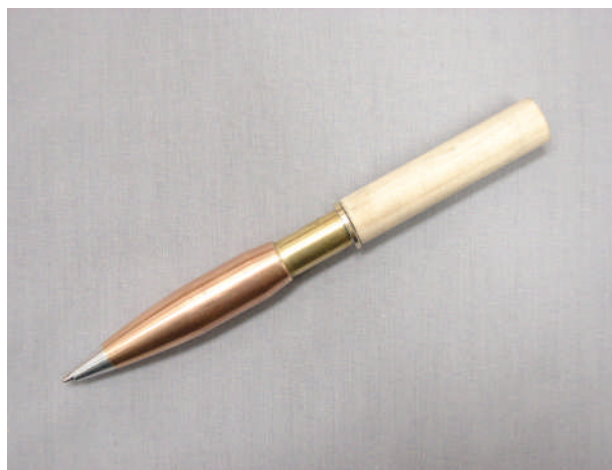
Dowel Insert Installed on Bullet Tip Assembly
