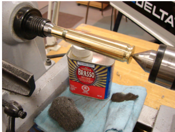
Polishing and Cleaning Between Centers
