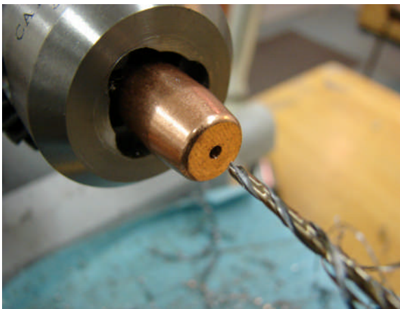
#36 Pilot Hole Drilled
