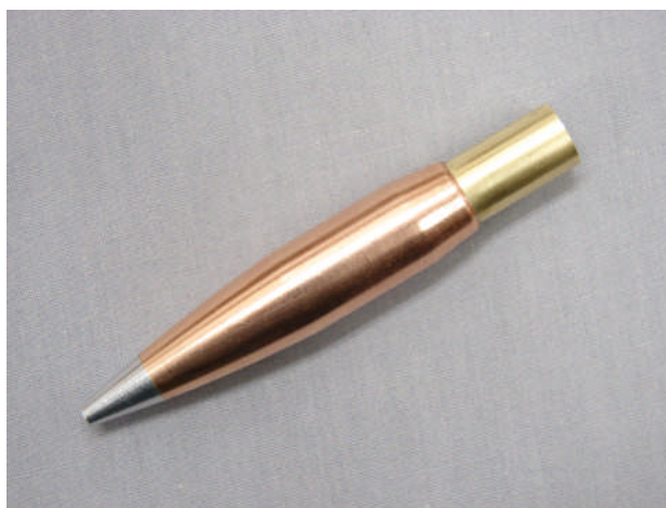
Tube Installed In Bullet With 22/32" Extension
