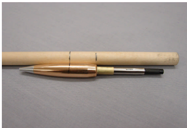
Cutting the Cross Dowel Insert to Length
