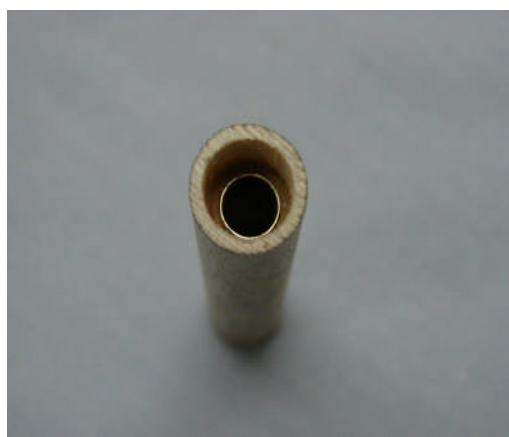
Insert With Tube Installed Flush
