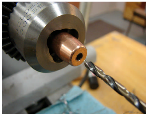
Drilled 9/64 Cross Refill Hole to 2-1/4"
