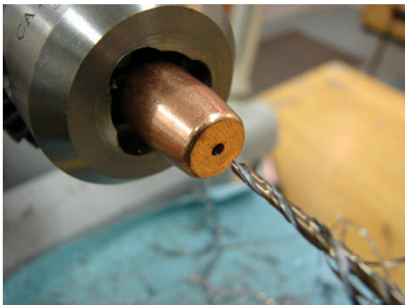
#46 Pilot Hole Drilled to a Depth of 1/2"
