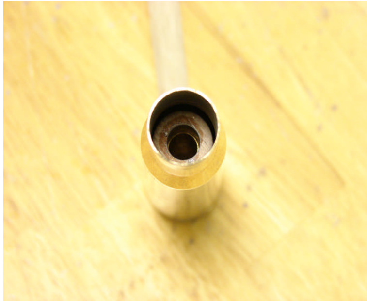
Dowel Insert Glued into Casing Bottom
