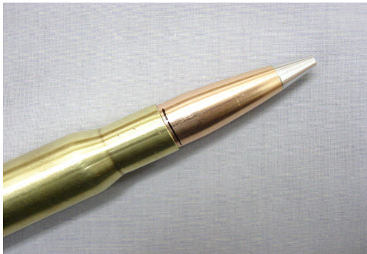
Mark the Bullet at the Casing Neck
