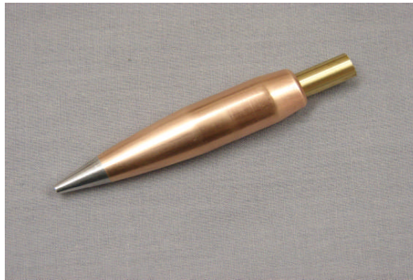
7mm Tube Installed In Bullet
