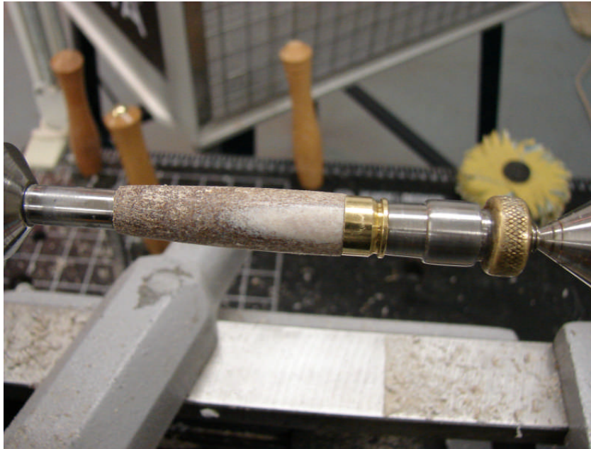
Antler Turned Down Using Cartridge Head As A Bushing
