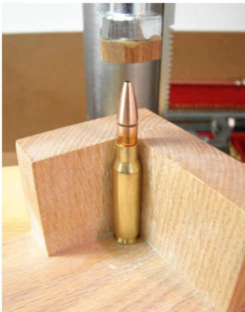
Seating Bullet Into Cartridge Neck
