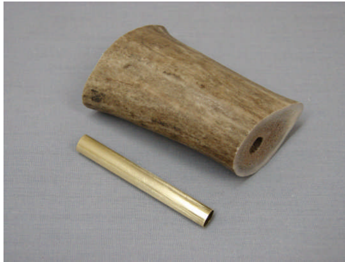
Antler Cut To Length Ready To Glue In Tube
