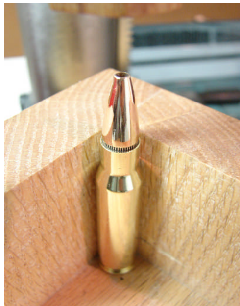
Seating Bullet Into Cartridge Neck
